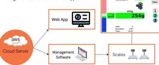
Operators can easily work with the led bar system as integrated in the touch screen controller, that indicates when a punnet is within the tolerance area and can be processed. The last stable end weight will be stored in the management software, making operator and weigh performance available for reporting and statistics.
